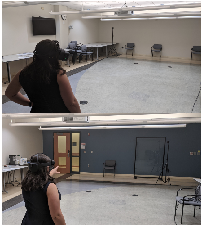
Figure 1: A participant estimating distances to virtual targets in both augmented reality HMDs. Visible on the floor are outlet covers; the virtual targets were not close to these.
