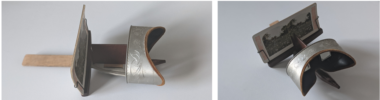
Figure 2.2: Antique stereoscope manufactured by Underwood & Underwood. The components are made of wood, aluminum, and brown velvet. The device was patented on June 11, 1901 in New York. Stereoscope courtesy of my dear friend Joe (Yuzhou) Huang.
