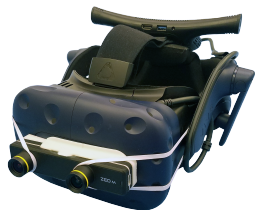
Figure 4.1: A VR HMD with VST capabilities: the HTC Vive Pro with mounted Zed Mini camera
