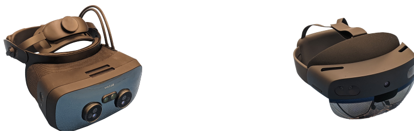
Figure 6.1: The optical see-through (OST) and the video see-through (VST) augmented reality display evaluated in Experiments 5 and 6. On the left is the Varjo XR-3 (VST AR) and on the right is the Microsoft HoloLens 2 (OST AR).
